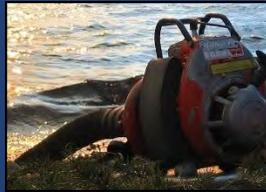
**Pumps**—once a water source is located crews can pump water to the fire. The most commonly used pump is a Centrifugal pump. The advantages of this type of pump for firefighting are: it has few moving parts, it is capable of pumping in-tandem with another pump, the water pressure can be changed by adjusting the RPM and they can be used in muddy water sources. While there are some disadvantages overall the pumps used are dependable.
