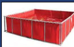
**Porta-Tanks**—porta-tanks are similar to relay tanks. These tanks are square and usually hold up to 4,500 litres (1000 gallons) of water. These tanks have a fabric liner that is affixed to a metal frame and is filled by tender, heli-bucketing, or by a pump relay system that pumps water into this holding tank. This system is somewhat cumbersome and would not be the first choice by crews.
