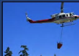
**Helicopters**—Helicopters are used a lot in suppression by bucketing on areas of a fire without manpower or areas too hot to safely deploy crews. There are times when crews will employ a bucket machine in mop-up. They will expose hot spots by grubbing them up allowing water to hit them directly when dropped from the air. This is an expensive application method and should only be used as a last resort.
