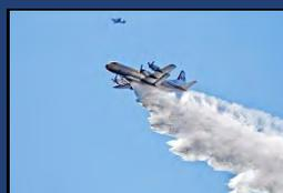
**Airtankers**—may be used to drop water or retardant. Airtankers are used to slow a fires forward movement or to cool a fire reducing fire behaviour. They are used to meet or support fire operations tactics and to support the crews on the ground.
